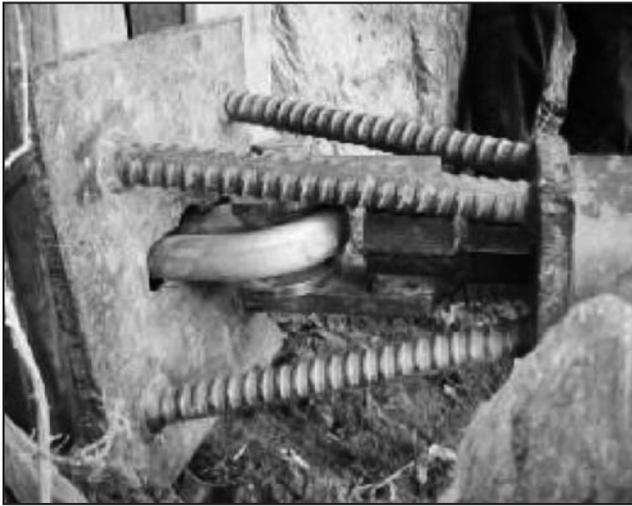
Figure 15. Anchor pull test
